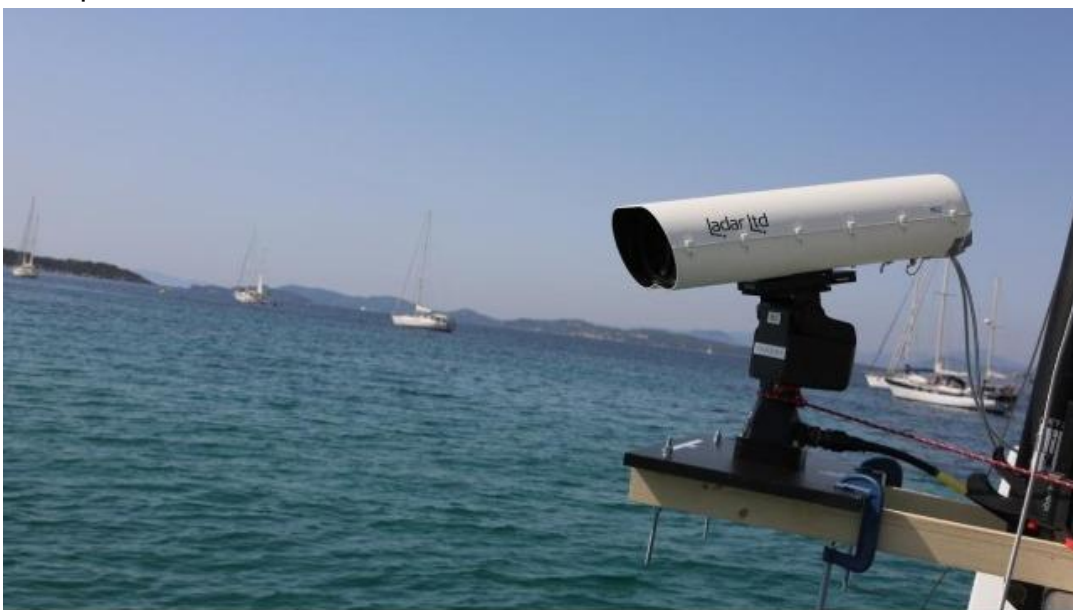
Compact Ladar installation on test vessel / Photo: Ladar Ltd
